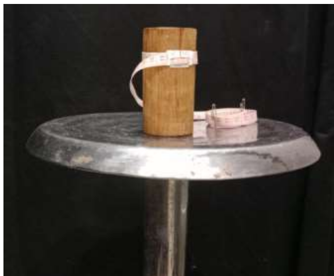
Fig. 4. Circumference of a cylinder obtained using tailor's tape (least count 0.005 cm)
