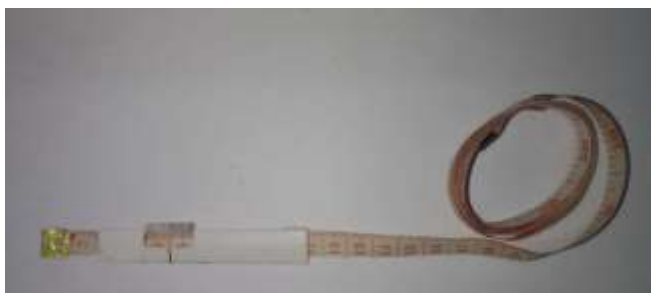
Fig. 3. Vernier-scale-based tailor's tape (least count 0.005 cm)
