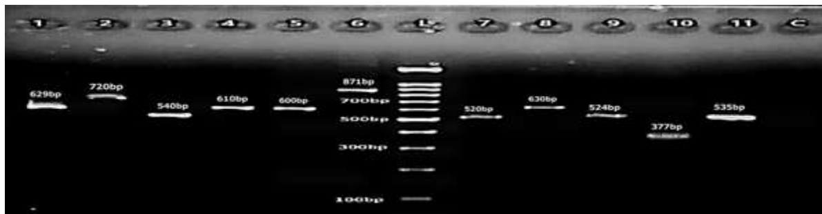
Fig. 2. Gel image of PCR-amplified products of the ITS regions of C. fabianii (1), C. kefyr (2), C. dubliniensis (3), C. guilliermondii (4), C. gattii (5), C. glabrata (6), the DNA ladder (100 bp), C. parapsilosis (7), R. mucilaginosa (8), C. tropicalis (9), C. lusitaniae (10), C. albicans (11) and the negative control (c).
